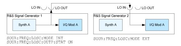
• Generation of 2x2 MIMO signal with one R&S Signal Generator, working in Coupled A->B mode.
